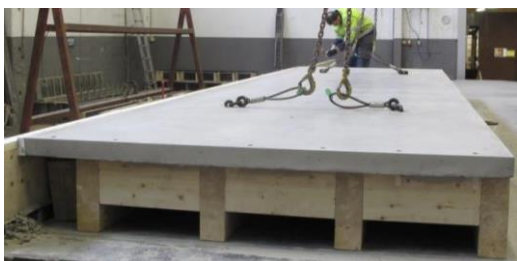
Figure 18: Timber-concrete hybrid floor. (Wålinder 2022)
