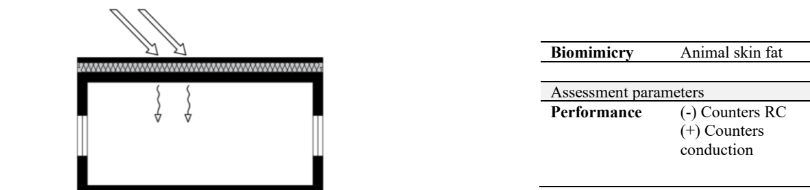
Figure 8: Left: Performance scheme of the insulated roof typology (Protective roofs). Right: Summary of the analyzed roof typology in terms of identified biomimetic role models and relevant assessment parameters.
