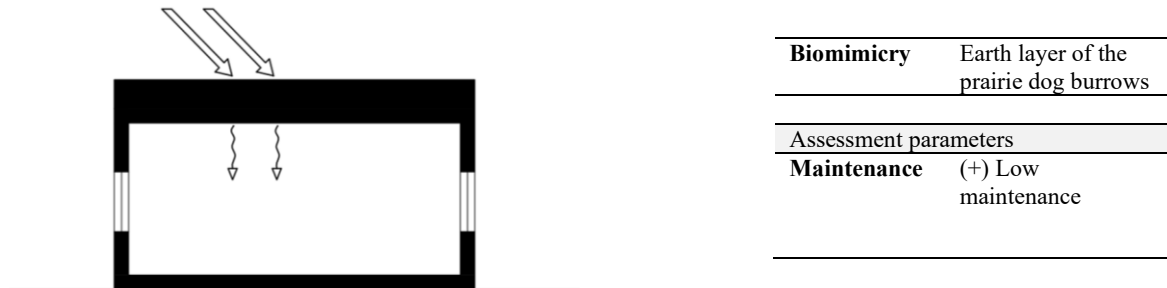
Figure 9: Left: Performance scheme of the Mass roof typology (Protective roofs). Right: Summary of the analysed roof typology in terms of identified biomimetic role models and relevant assessment parameters.
