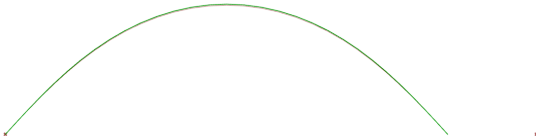
Figure 21 :Bending rod with karamba (green), and kangaroo2 (red), from a prescribed displacement
