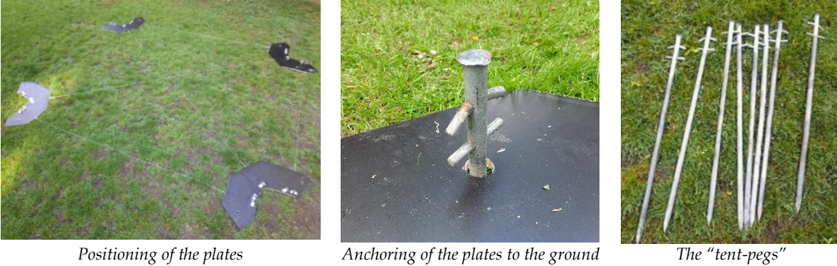
Figure 86 : Positioning then anchoring of the plates
