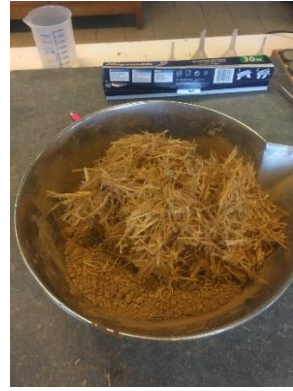
Figure 23: Straw after soil introduction (Personal picture)
