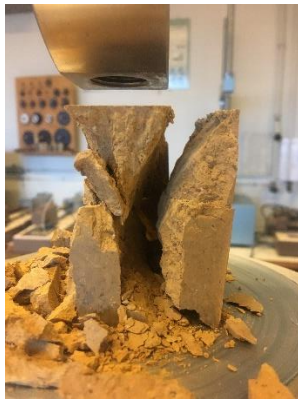
Figure 71: Unreinforced sample's failure planes 1
