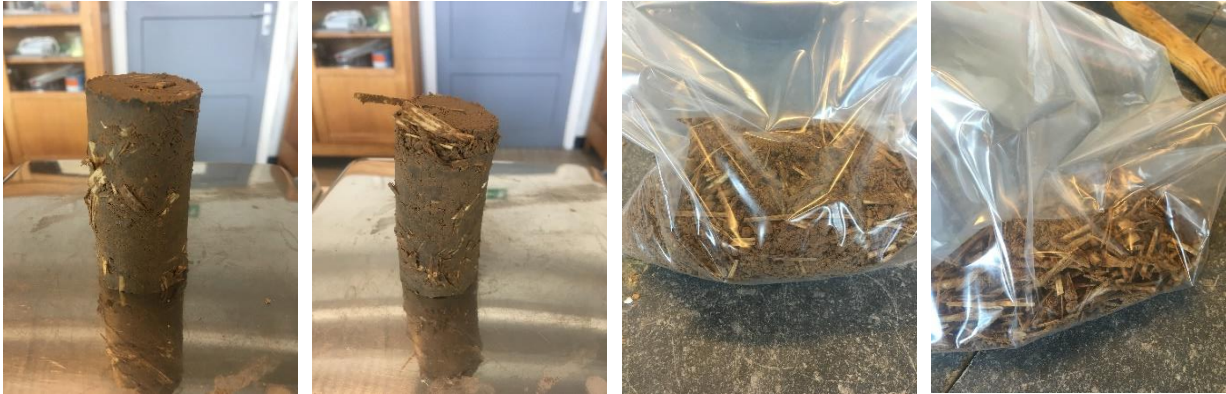
Figure 32: Sample P, 20% straw: Deformation 1 (Personal picture)
