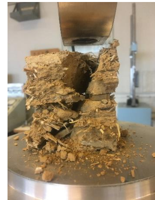
Figure 74: Reinforced sample's failure plane 2
