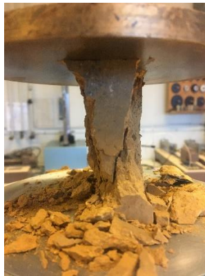
Figure 72: Unreinforced sample's failure plane 2
