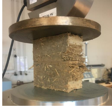
Figure 59: Greased contact surfaces (Personal picture)
