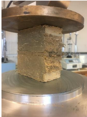
Figure 65: Regular contact area (Personal picture)
