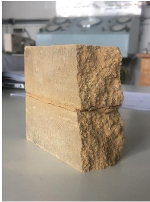
Figure 64: Irregular contact area (Personal picture)
