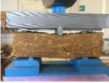
Figure 54: Failure under shear stress (Personal picture)
