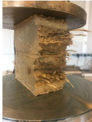
Figure 66: Irregular contact area (Personal picture)
