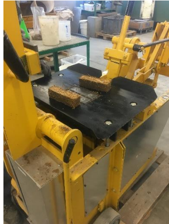
Figure 45: CEB compaction (Personal picture)
