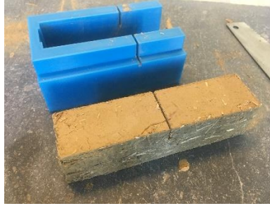
Figure 55: Failure initiation gap (Personal picture)
