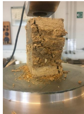
Figure 73: Reinforced sample's failure plane 1
