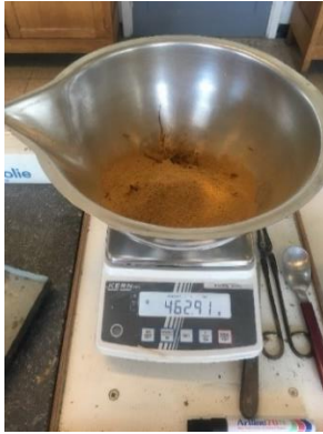
Figure 21: Soil after straw introduction (Personal picture)
