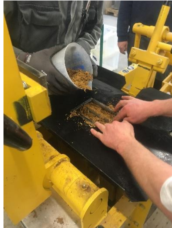
Figure 44: CEB moulds filling (Personal picture)
