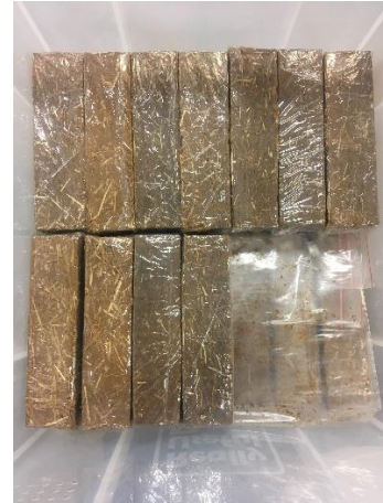
Figure 46: Hermetical stacking of CEBs (Personal picture)
