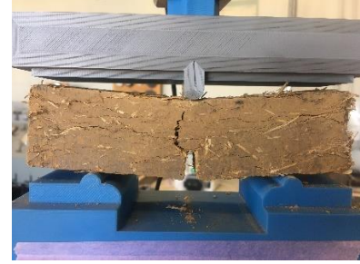
Figure 56: Failure under flexural stress (Personal picture)
